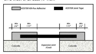
Do not stress the system for at least 24-48 hours after application. Protect the freshly applied system from water, rain and frost until it is fully cured.
