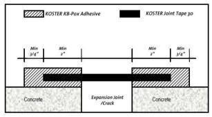
Do not stress the system for at least 24 - 48 hours after application. Protect the freshly applied system from water, rain and frost until it is fully cured.
