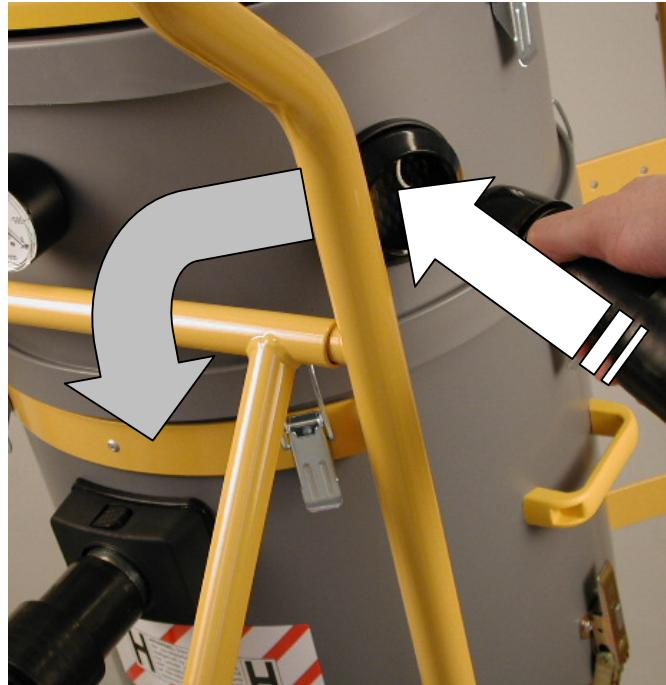
At the same time fresh air floats the opposite way through the tube filter in order to balance the pressure in the dust container and in the hose.
