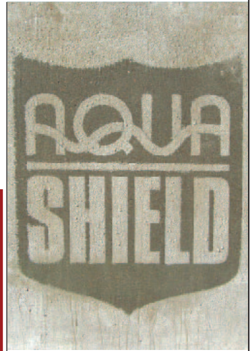
In the photo above, a concrete slab was treated with Ameripolish® AquaShield™ Waterproofing Treatment, all except the 'shield' outline, which was masked off and remained untreated. When sprayed with water, the untreated section absorbed water and turned dark. Water beaded up on the AquaShield treated area, and it looks completely dry.
